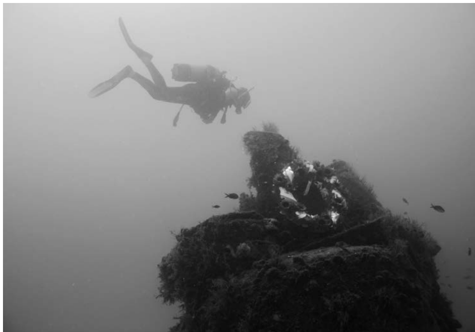
FIG. 19. The Scirè tower after the damage done in 2002, with the periscope masts broken (F.R.).
